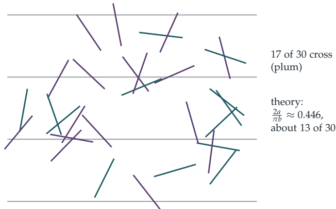
Figure 12.20.1 Thirty needles of length 2a = 1.4 thrown onto lines 2b = 2 apart. The ones crossing a line are plum. Here 17 cross, compared with the 13.4 expected: small samples give rough estimates, and Buffon's needle is a famously slow way to compute \pi .
